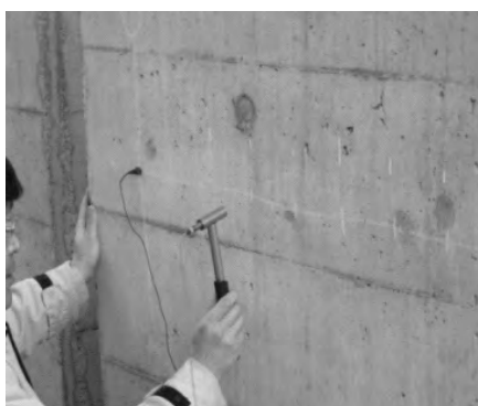
Fig. 16 Impact-echo testing at Odawara fishing port.
